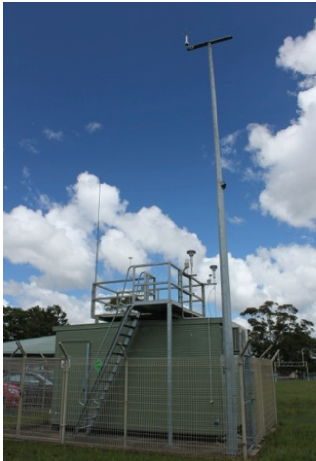
Figure 3: Office of Environment and Heritage air quality monitoring station at Beresfield (Source: NSW Minerals Council)
