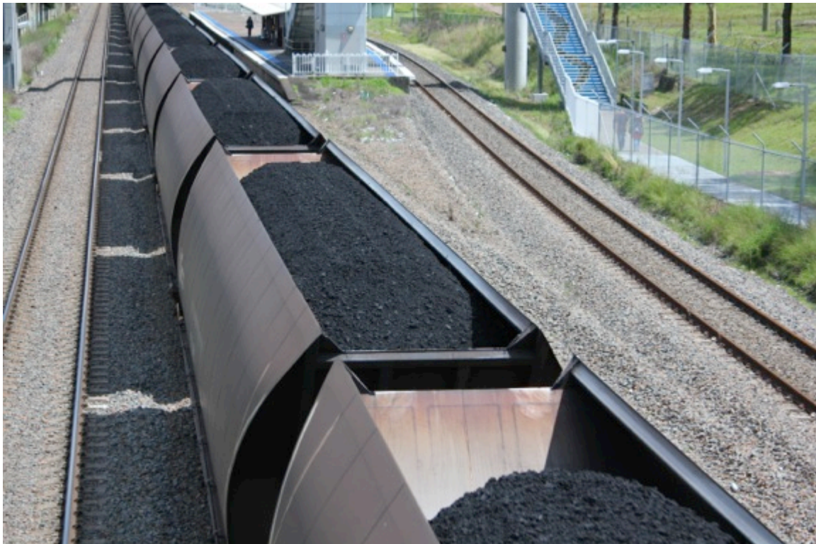
Figure 6: Coal loads on the Main North Rail Line showing an even, consistent surface profile (Source: NSW Minerals Council)
